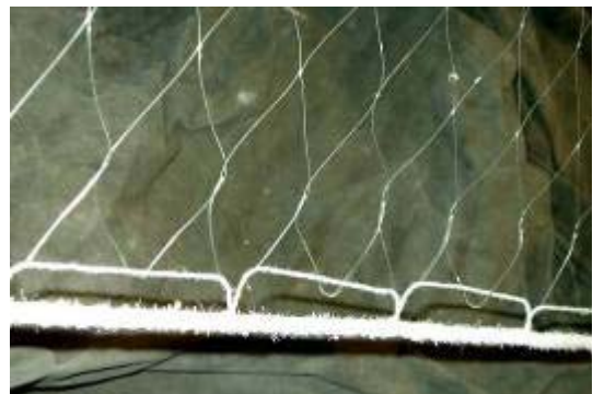
Figure 3b: Net that has been slung correctly to ensure optimal catching efficiency
