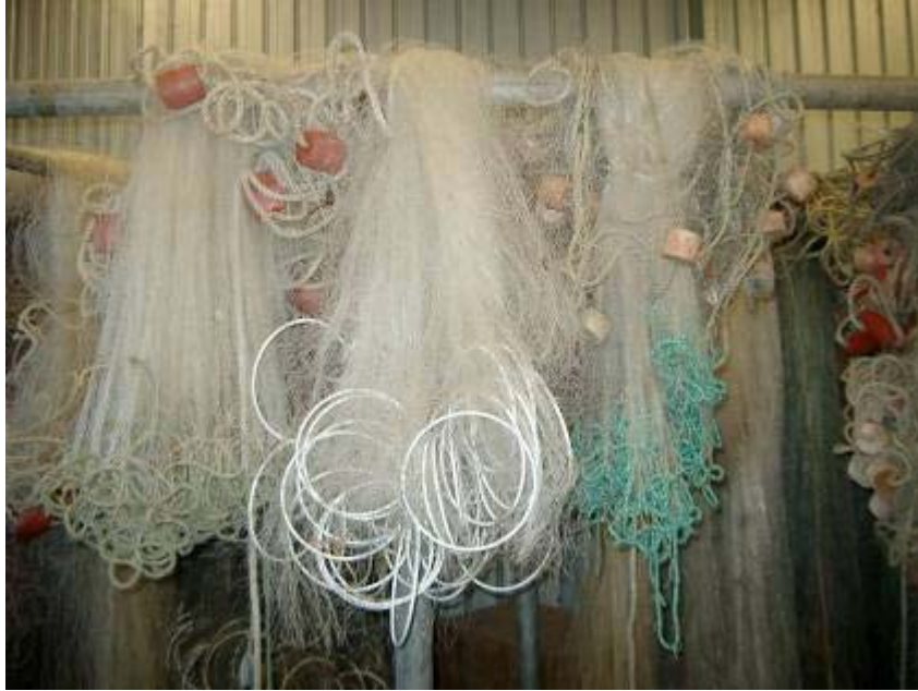
Figure 4. Ring net (shown middle); an alternative to the use of lead line. Suitable for calm conditions
